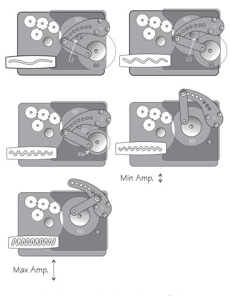
Amplitude may be changed in any of the patterns by moving the crank connection to a different hole.
